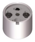
Humidity reference cells, also known as "salt pot" in the past, serve to control and adjust the humidity probes. The cell will be produced in testing chambers attaining a highly defined relative air humidity by using a saturated salt solution. Exact calibrations are now possible when using the reference cells between the sensor and reference humidity in the styropor insulation container.
