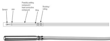
However, depending on the requirements, this simple execution of temperature measurement also reaches its limits. Although the cable probes can be cast waterproof up to a maximum permanent temperature of approx. 350 °C, there is still the possibility that water vapor could get inside the probe. Particularly when using glass fiber lines, which are used at high ambient temperatures (>260 °C), moisture can penetrate the measuring insert and impair its function.
