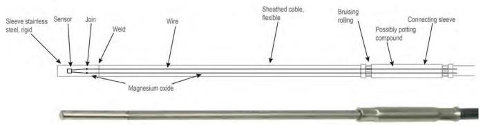
All these advantages and properties mean that significantly more and higher quality basic materials are required for a mineral insulated resistance thermometer. The manufacturing processes are also more complex, which means that the price is higher than that of a simple cable probe. In comparison to a high-quality cable probe (with R glass fibre cable), there is almost no difference in price.
